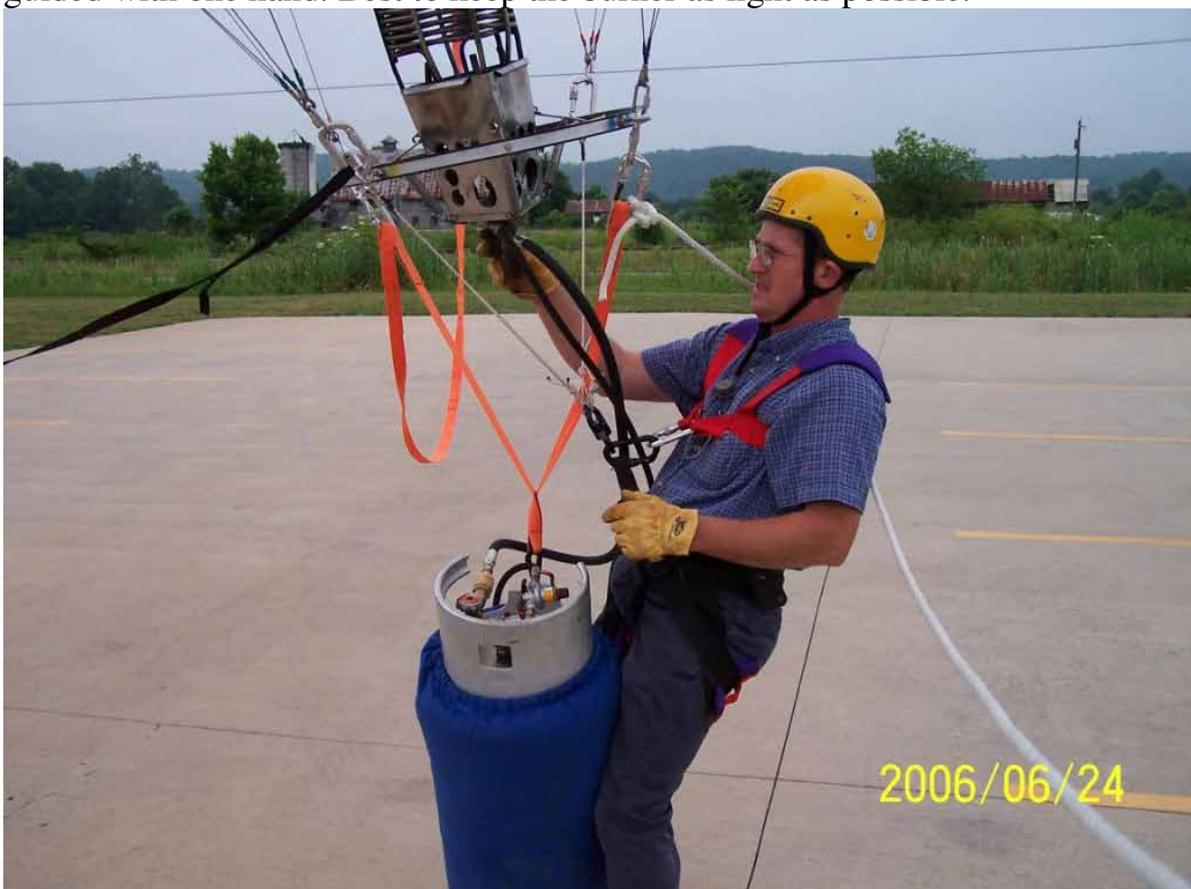
There are distinct disadvantages of flying a non-rigid suspension system and one must be aware of flying conditions and environment when using such a system. The advantages allow portability (easy to transport and store) and flexibility (fuel tanks and burners are easy to change) with minimum weight.
