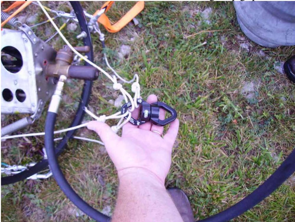
**Kev-cord** - Kevlar core rated at 1850 pounds break and is flame resistant. This Kevlar based cord allows the lines to be knotted and adjusted while still allowing a 900 pounds break strength even allowing for the knots decreasing
