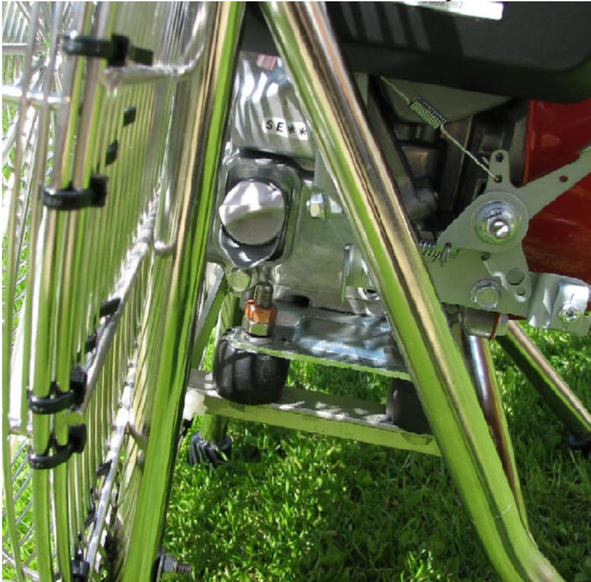
Note here, the positioning of the oil fill/drain points are towards the top of the "V" in the frame, so not all will find it easy to get to, you may need a pair of pliers to turn the cap!!.
