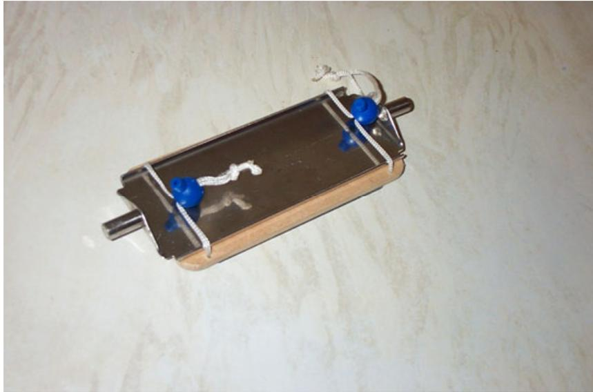
Tim says, "I mounted a mirror on a piece of wood which then attaches to the Lindstrand steel mirror. If you use two mirrors you can see the tank gauge the correct way round."
